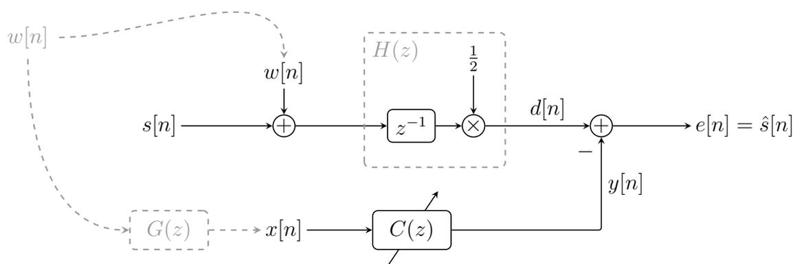
A speech signal  $s[n]$  (for simplicity, it is assumed that  $s[n]$  is a white Gaussian noise signal with unit variance) is superimposed with statistically independent white Gaussian noise  $w[n]$  with some variance  $\sigma_w^2$ . Unfortunately the noise reference is filtered by an IIR-filter  $G(z)$  before it is captured. The filter is specified by the purely recursive difference equation
