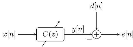
We want to design a filter according to some specifications with the help of the Wiener-Hopf equation. To this end, we assume that the input signal  $x[n]$  is given as
