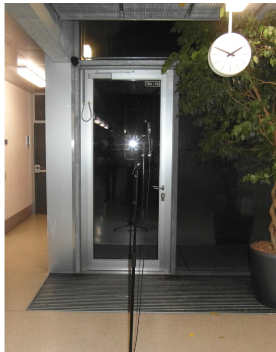
Figure 4.5: Example of source and microphone positioning
