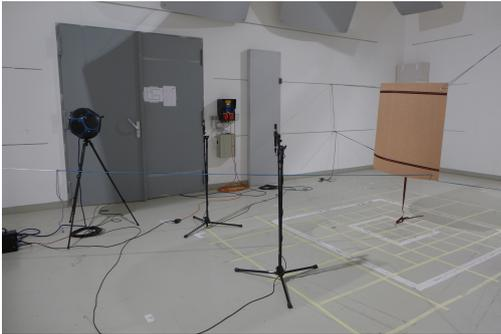
Figure 1: Measurement setup in the reverberation chamber
