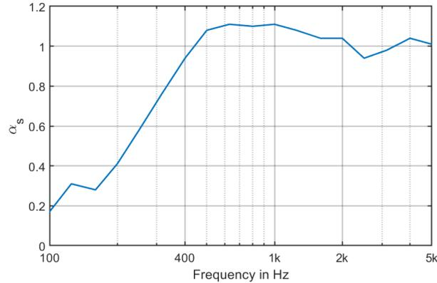
Figure 2.4: Statistical absorption coefficient  $\alpha_s$  over frequency for the same PET absorber material found in the HVB, but at a larger thickness of 50 mm [10].
