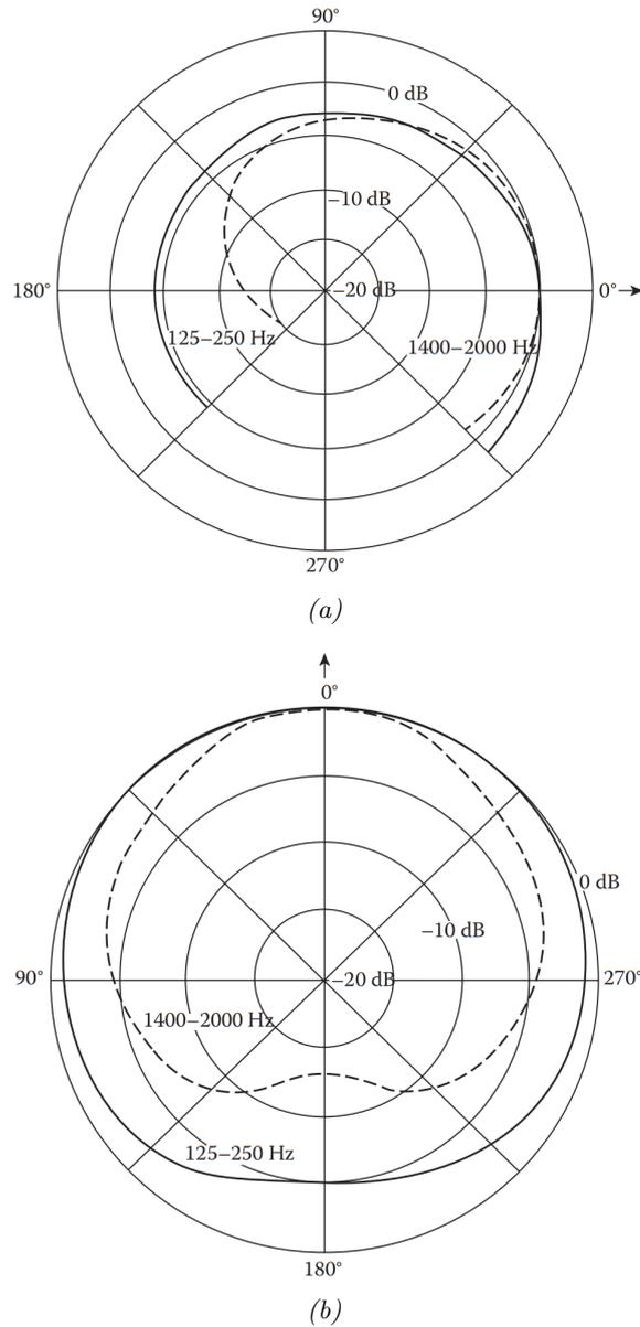
Figure 2.1: Directionality of the human voice in the vertical plane (a) and in the horizontal plane (b) [3].
