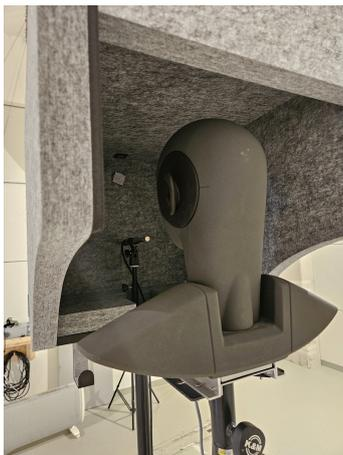
(a) Measurement microphone, artificial head with HVB
