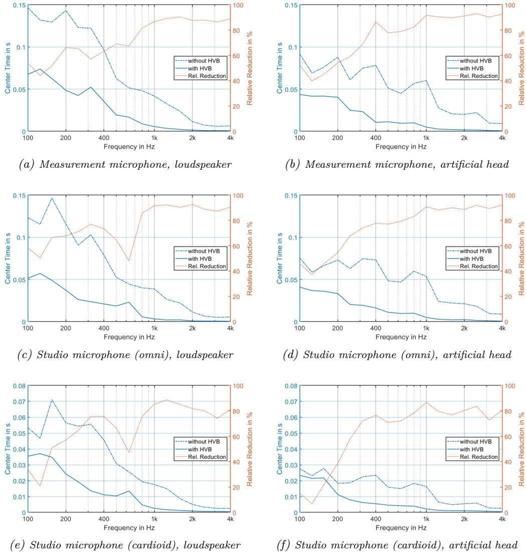
Figure 3.8: Center Time  $T_c$  in seconds with the HVB (blue) and without it (blue, - - -), evaluated in 1/3-octave bands. Relative Reduction due to the HVB is also given (orange, ···).
