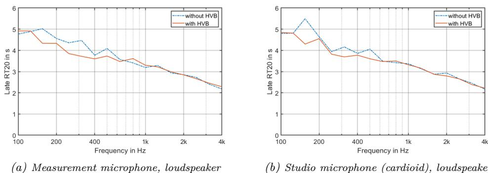
Figure 3.6: Late reverberation time  $RT_{20}$ , taking into account a level-drop of 20 dB in the respective third-octave band of the  $EDC$  starting from 40 ms after the start of the  $EDC$ . Late  $RT_{20}$  was calculated without the HVB (blue) and with the HVB (orange). Used equipment were the loudspeaker, the measurement microphone (left), and the studio microphone (right).
