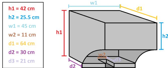
Figure 2.3: Inner dimensions of the *t.akustik Vocal Head Booth*
