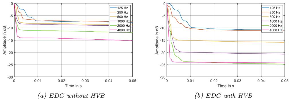
Figure 3.5: First 50 ms of the Energy Decay Curve  $EDC$  using the studio microphone (cardioid) and the loudspeaker without the HVB (left) and with the HVB (right). The  $EDC$  is evaluated in octave-bands from 125 Hz to 4 kHz.
