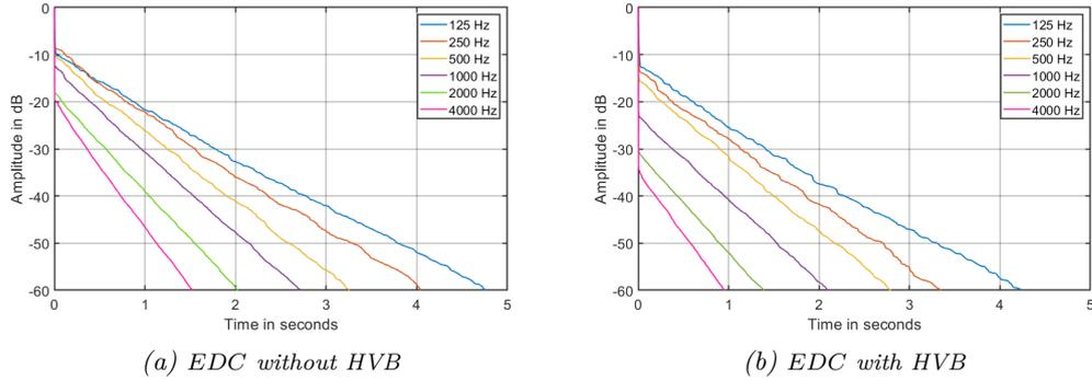
Figure 3.4: Energy Decay Curve  $EDC$  using the studio microphone (cardioid) and the loudspeaker without the HVB (left) and with the HVB (right). The  $EDC$  is evaluated in octave-bands from 125 Hz to 4 kHz.
