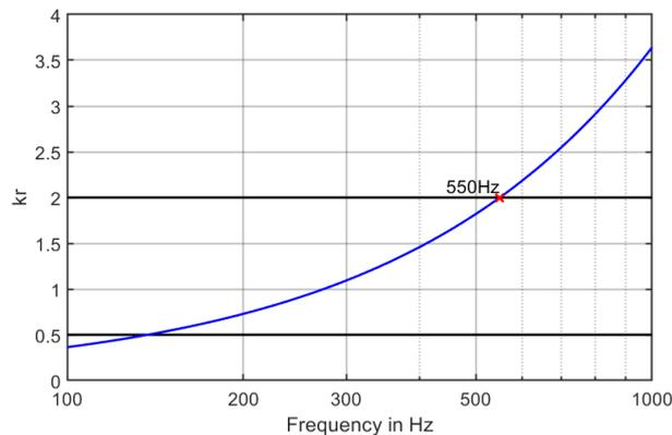
Figure 2.5:  $kr$  over frequency  $f$  at a distance from the source  $r = 20$  cm. The two thick black lines indicate the borders between near-field, transition region, and far-field (from bottom to top)
