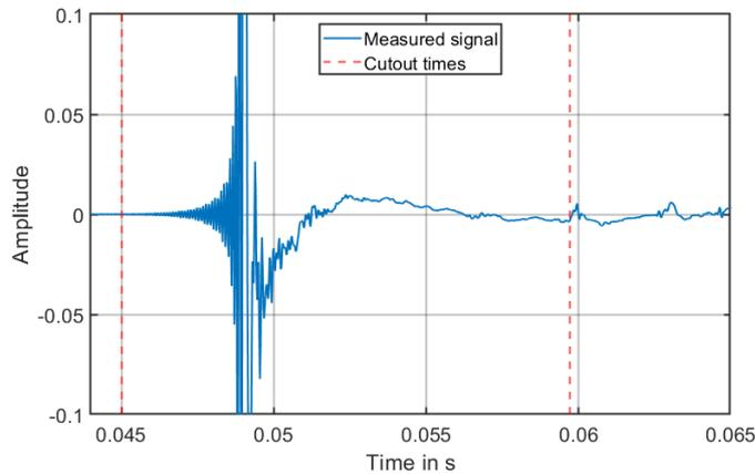
Figure 3.2: Start of impulse response measured in reverberation chamber with Measurement microphone and loudspeaker, but without HVB. Cutout times are marked.
