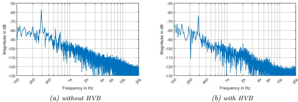
Figure 4.1: Frequency response of background noise and hum calculated from the recorded example.
