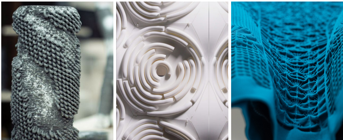
(a) Novel 3D printing material [Utrecht, 2023]. (b) Compact sound absorber addressing lower frequencies, 3D printed [Setaki et al., 2023]. (c) Double layered textile sound barrier, knitted and stitched [sound barrier, 2023]
