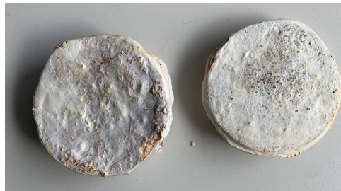
Figure 3.2: Porous sample of a foam made of mycelium and sawdust.
