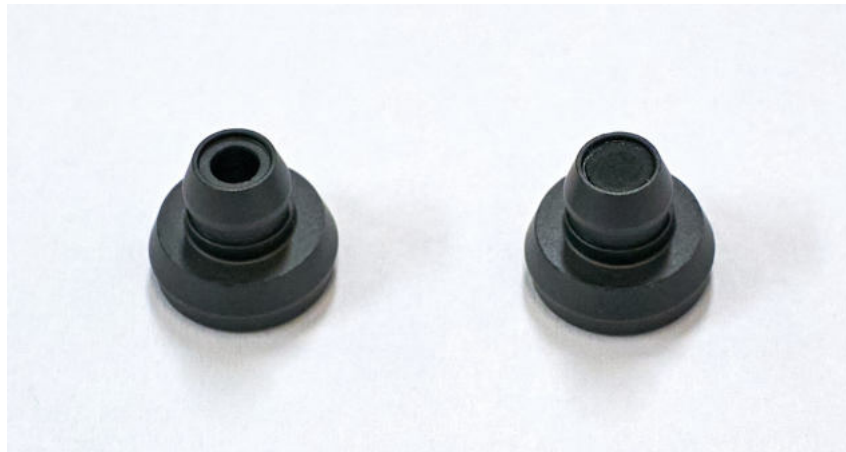
Figure 3.15: headphone prototype without (left) and with (right) fleece
