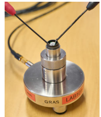
(b) contacted headphone in in-ear adapter on the ear simulator
