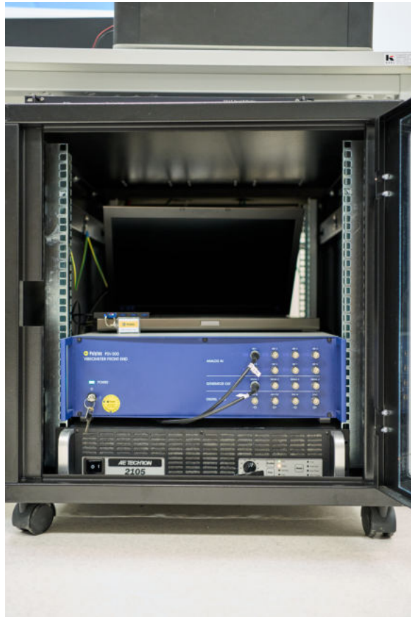
(b) computer, front end and amplifier used for the measurement
