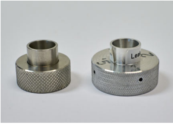
(a) GRAS RA0088 in-ear adapter (left) and special made leakage adapter (right)
