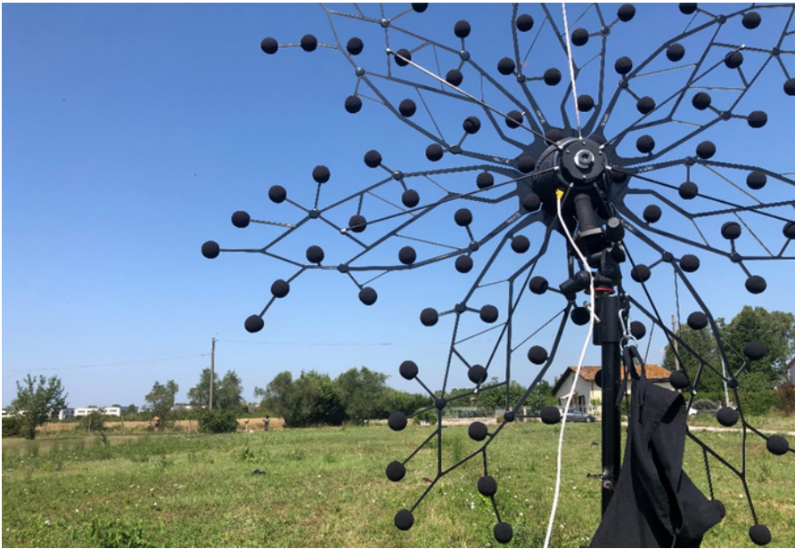
Figure 2.2: Acoustic camera in the free field setup before conducting the performance test under the different conditions.
